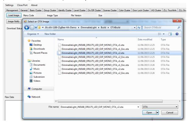
After loading the binary file, the ZGWUI will populate the Load Image textboxes with some useful data, including manufacturer code, image type, file version and binary size.
